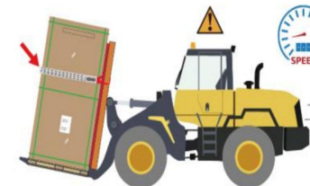
When transporting by truck, the packaging box must be tilted against the forklift gantry and the components must be fixed to the forklift with a safety rope with a tensile strength of >2000kgf, and the speed must be controlled to prevent tipping.
